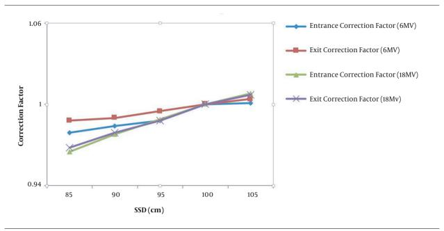
Figure 3. SSD correction factor for entrance and exit diode types for 6MV and 18MV photon beams
