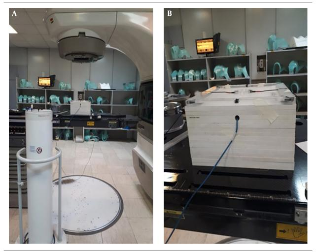
Figure 1. A, Illustration of diode system and Linac for in vivo dosimetry; B, Setup for determination of the calibration factor for entrance point by ion chamber
