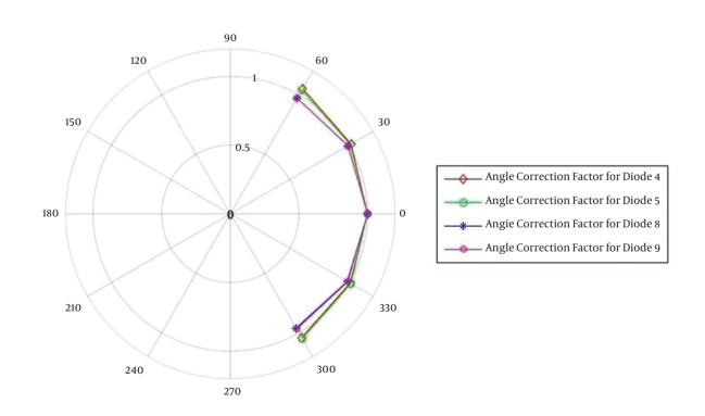
Figure 4. Angle correction factor for different diode detectors
