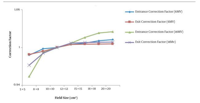
Figure 2. Field size correction factor for entrance and exit diode types for 6 MV and 18 MV photon beams
